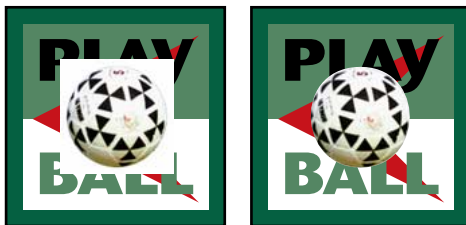
Image imported into Illustrator without image clipping path, and with image clipping path
